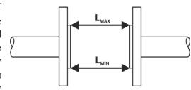
The opposition of the holes in the counter-flanges for the bolts should be ensured in the same manner and a sufficient room behind the flanges should be available for the bolts and nuts so that the actual installation of the sensor in pipeline and its attachment with the bolts is made possible.
