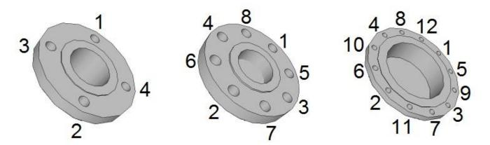
If the bolts are tightened too much during the installation of pipework components, deformation of the sealing surface may occur. In consequence, the torque values indicated in the table are used as a guidance for tightening the screws and bolts.
