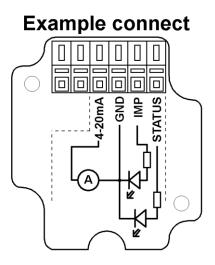
The maximum frequency of the pulse output is 1,6kHz when pulse width min. 250µs
